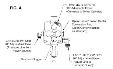
Connect the <sup>3</sup>/<sub>4</sub>" I.D. x 24" long hose from the control valve work port to the Post Driver hydraulic cylinder port.
